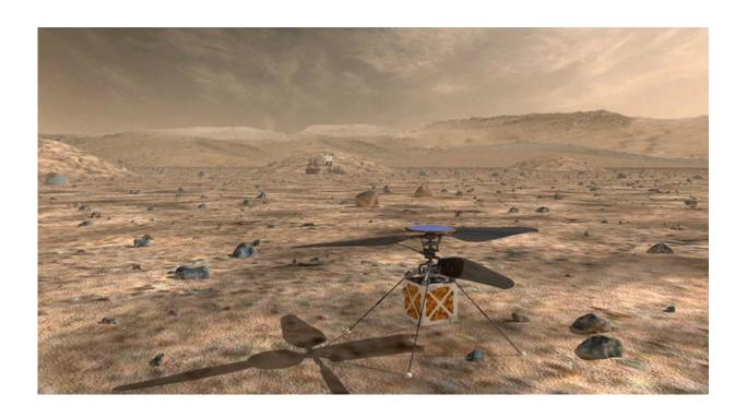
The Mars Helicopter, a small, autonomous rotorcraft, will travel with NASA's Mars 2020 rover, currently scheduled to launch in July 2020, to demonstrate the viability and potential of heavier-than-air vehicles on the Red Planet. Credit: NASA/JPL-Caltech
