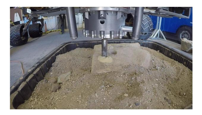
A test of a new percussive drilling technique at NASA's JPL. Later this week, NASA's Curiosity rover will test percussive drilling on Mars for the first time since December 2016. Credit: NASA/JPL-Caltech
