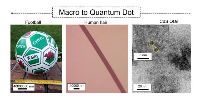
A size comparison in nanometres of a football, human hair and quantum dots, which are less than 10 nanometres. Credit: S Pitchaimuthu, Swansea University
