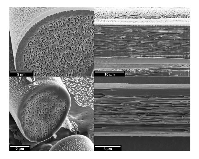
Scanning electron micrographs of man-made fibers emulating the optical properties of comet moth cocoon fibers. Top row: Transverse and longitudinal cross-sections, respectively, of a synthesized fiber made of regenerated silk containing a high density of filamentary air voids. Bottom row: Corresponding images of a PVDF (polyvinylidene difluoride) fiber containing a high density of filamentary voids. Credit: Norman Shi and Nanfang Yu/Columbia Engineering
