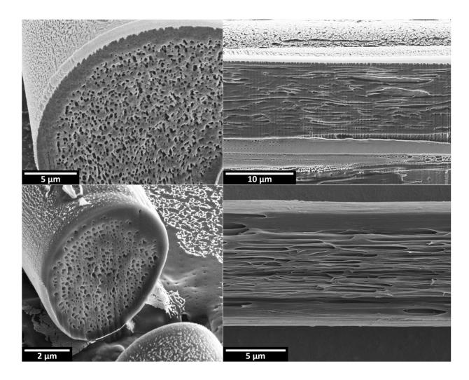
Scanning electron micrographs of man-made fibers emulating the optical properties of comet moth cocoon fibers. Top row: Transverse and longitudinal cross-sections, respectively, of a synthesized fiber made of regenerated silk containing a high density of filamentary air voids. Bottom row: Corresponding images of a PVDF (polyvinylidene difluoride) fiber containing a high density of filamentary voids. Credit: Norman Shi and Nanfang Yu/Columbia Engineering
