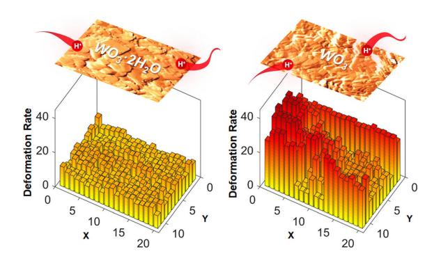
AFM reveals that structural water in tungsten oxide results in smaller deformation rates from ion intercalation, an unexpected finding on the role of structural water that can enable materials with higher power and efficiency energy storage devices. Credit: North Carolina State University
