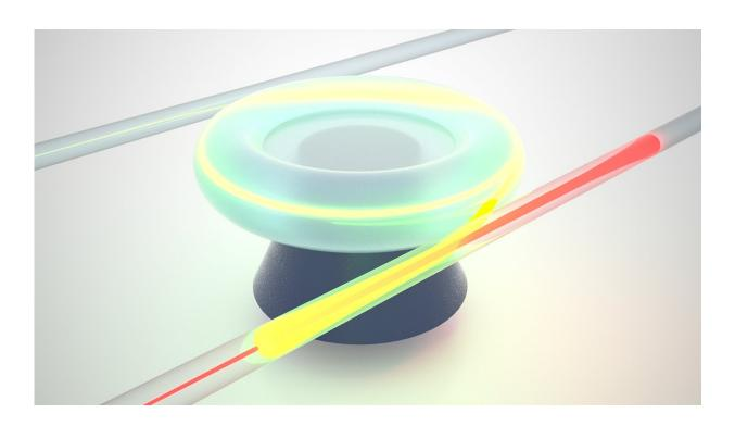
Artist impression of the light circulator. The yellow beam enters at the upper left port and is forced to leave the resonator at the lower left port. The red beam enters at that port (lower left) but cannot follow the reverse path of the yellow beam as it is forced to propagate to the lower right exit. Credit: Henk-Jan Boluijt (AMOLF)
