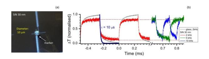
(a) Video still showing a tightly focused laser beam making contact with the thermocouple. (b) Graph showing the thermocouple's response over time to different laser powers (3.6 and 1.8 mW) at different repetition rates, on glass and on the silicon nitride membrane ( $\Delta$ T: change in temperature,  $\tau$ : time for temperature rise and decay). Credit: *Scientific Reports*
