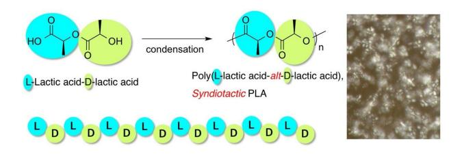
Method for synthesizing 'pure' syndiotactic poly(lactic acid) polyesters and picture of spherulite thereof. Graphical Abstract of *Polymer Chemistry*, 2018, 9, 2446-2457. DOI: 10.1039/C8PY00391B-Reproduced permission of The Royal Society of Chemistry. Credit: Toyohashi University of Technology. All Rights Reserved.
