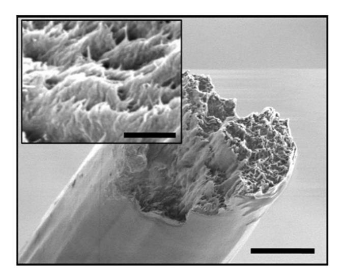
SEM image of the cross-section of the fibre, showing the aligned nanofibrils. Credit: KTH The Royal Institute of Technology
