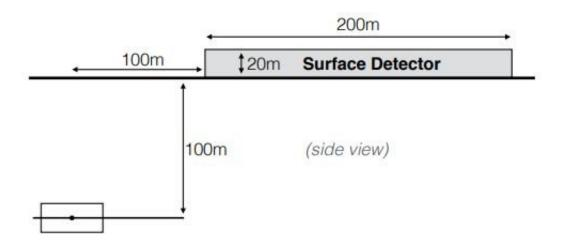
Possible geometric configurations for the MATHUSLA surface detector at the HL-LHC. Gray shading indicates areas assumed to be sensitive to LLP decays. The surface detector is a 200m square building, centered along the beam line. Credit: arXiv:1606.06298 [hep-ph]
