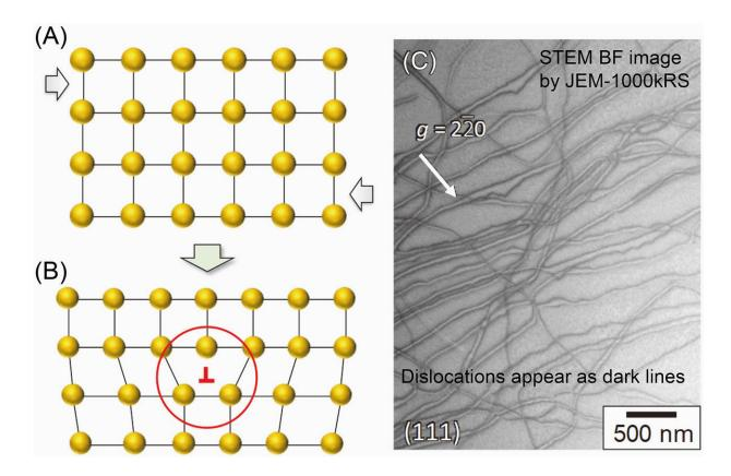
Plastic deformation of materials is caused by nucleation and multiplication of dislocations under an external force (A and B). It is generally believed that brittle inorganic semiconducting materials have difficulty in formation of dislocations due to their strong chemical bonds. However, we found that a great number of dislocations are generated and multiplied in ZnS crystals during deformation in darkness (C), resulting in the extraordinary plasticity. Credit: Atsutomo Nakamura
