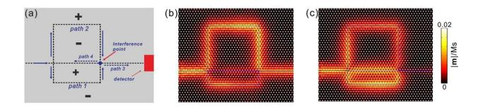
Illustration of the magnon interferometer with interference patterns. Credit: Li et al. ©2018 American Chemical Society
