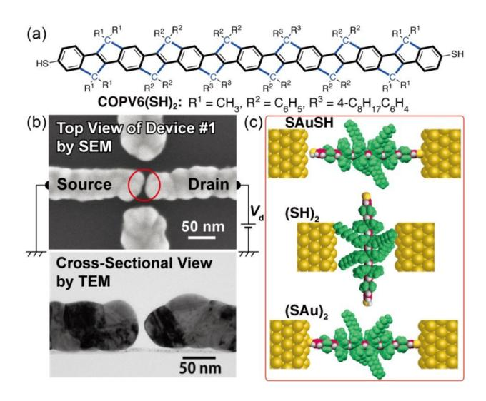
(a) Molecular structure of the COPV6(SH)<sub>2</sub> molecule. (b) Top and cross-sectional views of an ELGP nanogap electrode. (c) Different ways in which the molecule binds with the nanogap. The thermally stable device is obtained when the first type of binding (SAuSH) occurs. Credit: *ACS OMEGA*
