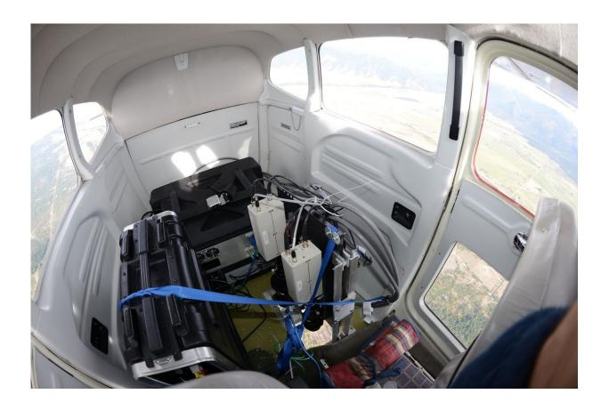
The LiDAR instrument aims a laser beam downward through a hole in the bottom of the plane. The beam was angled backward so that the light's reflection on the water is deflected away and does not saturate the receiver. Credit: Joseph A. Shaw, Montana State University
