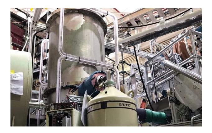
The UNCtau 'bottle' trap. A combination of magnetic fields and gravity prevent neutrons from escaping the container. Credit: Los Alamos National Laboratory
