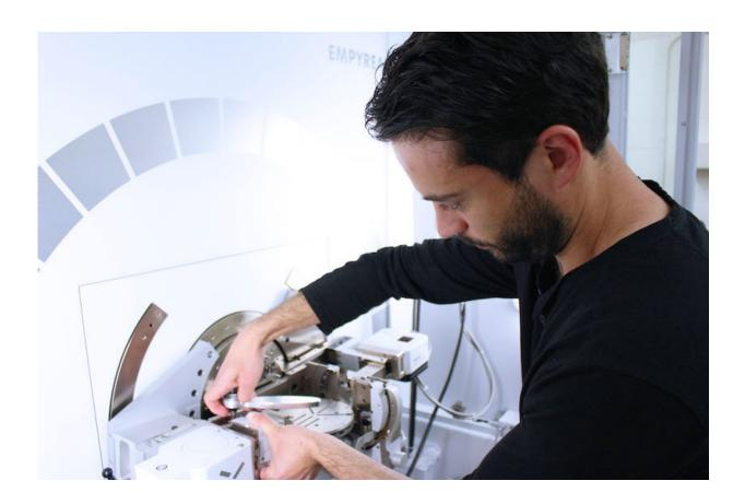
Postdoctoral scholar Anastasios Pateras adjust an X-Ray instrument used to detect previously unknown defects in quantum dots. Credit: Sam Million-Weaver
