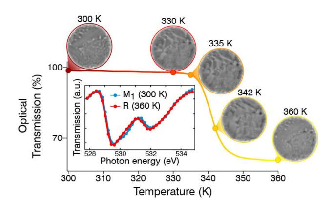
Phase transition from insulator to metallic phase in VO2 as a function of the temperature. Credit: ICFO
