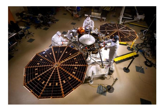
The solar arrays on NASA's InSight lander are deployed in this test inside a clean room at Lockheed Martin Space Systems, Denver. This configuration is how the spacecraft will look on the surface of Mars. Credit: NASA/JPL-Caltech/Lockheed Martin
