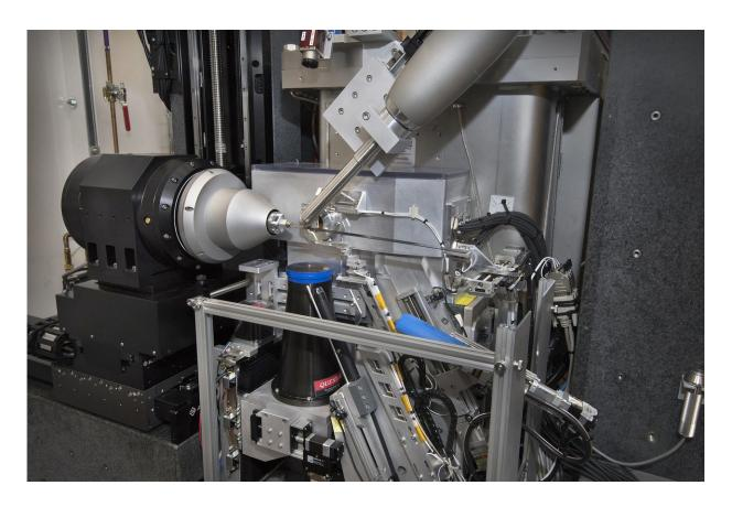
The new goniometer scanner system will soon be available to the FMX beamline's general user groups, and will open a pathway to structure determination from crystals smaller than ever before. Credit: Brookhaven National Laboratory
