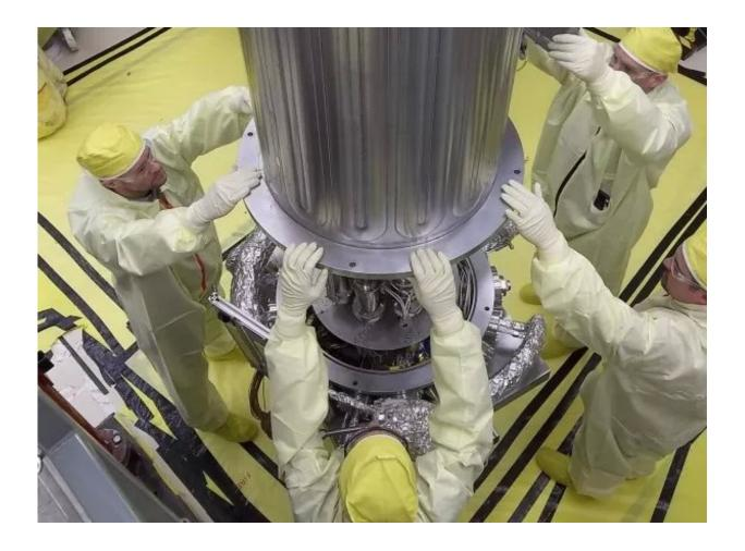
NASA & National Nuclear Security Administration (NNSA) engineers lower the wall of the vacuum chamber around the KRUSTY system at the Nevada National Security Site (NNSS). Credit: Los Alamos National Laboratory
