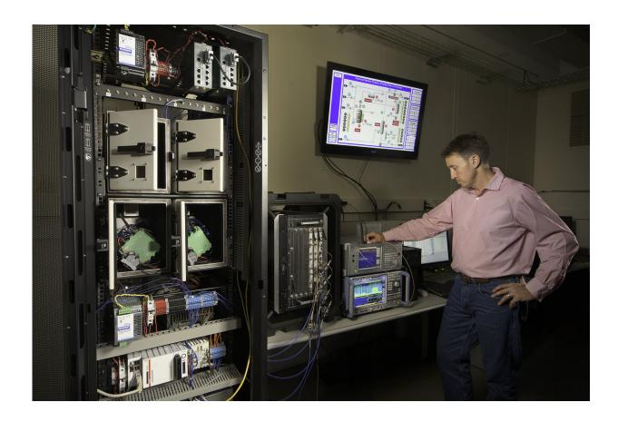
Using a novel testbed that recreates factory environments in the lab, NIST engineer Rick Candell helps 'cut the cords' (and wires) from industrial communications networks by studying how different factory layouts affect wireless radio frequencies, and in turn, how this impacts factory performance. Credit: Earl Zubkoff
