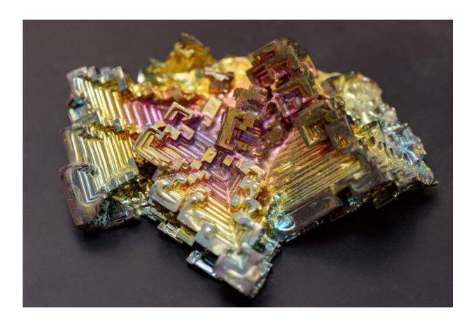
This is bismuth. UD researchers have identified a specialized capability in the metal, called "catalytic plasticity," that can be harnessed to convert carbon dioxide into liquid fuels and industrial chemicals. Credit: University of Delaware
