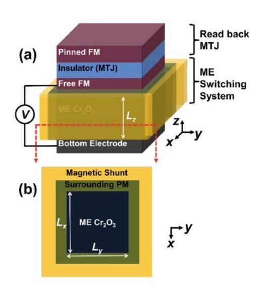
(a) side and (b) overhead views of the proposed switching element show the
