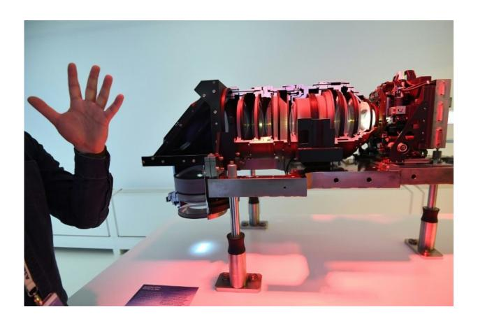
A lens used in the manufacturing of semiconductors at Dutch company ASML, whose latest systems project blueprints of circuitry onto silicon wafers
