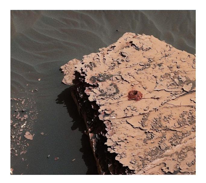
NASA's Curiosity rover successfully drilled a hole 2 inches (5.1 centimeters) deep in a target called "Duluth" on May 20, 2018. The hole is about .6 inches
