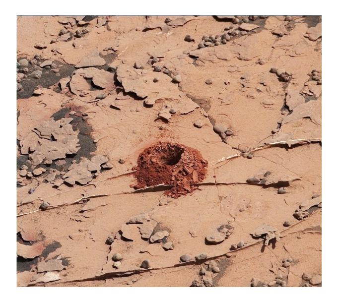
A close-up image of a 2-inch-deep hole produced using a new drilling technique for NASA's Curiosity rover. The hole is about 0.6 inches (1.6 centimeters) in diameter. This image was taken by Curiosity's Mast Camera (Mastcam) on Sol 2057. It has been white balanced and contrast enhanced. Curiosity drilled this
