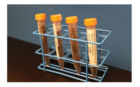
Human hair samples provide the instrument calibration standard for the new technique. Credit: Manuel Kleiner.
