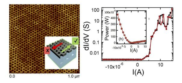
The left shows the atomic force micrograph, exhibiting honeycomb structure pattern behind a magnetic device. Inset shows the schematic of current flow direction. On the right: electrical data reveals diode-type behavior of current flowing in one direction. Inset shows that the dissipative power is of the order of nano-watt in the current flowing direction, which is at least three orders of magnitude smaller than the semiconductor diode. Credit: Deepak Singh
