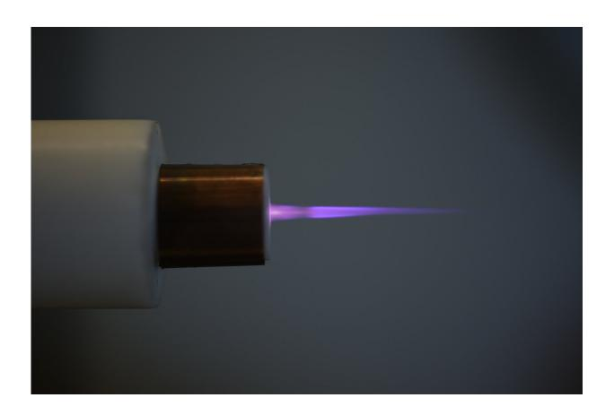
Purdue researchers have developed a new device that generates cold plasma and could transform how medical tools are sterilized. Credit: Purdue University
