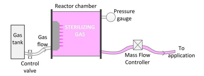
Purdue researchers have developed a method to use DC voltage cold plasma technology to produce a sterilizing gas for medical device packaging. Credit: Purdue University
