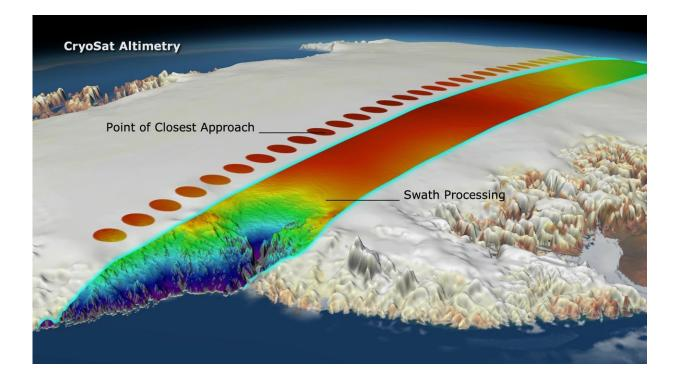
The technique of swath processing differs from conventional radar altimetry. Using CryoSat's novel interferometric mode, whole swaths, rather than single points, of elevations can be computed. This is yielding more detail that ever before on how glacial ice is changing. Credit: ESA/Planetary Visions
