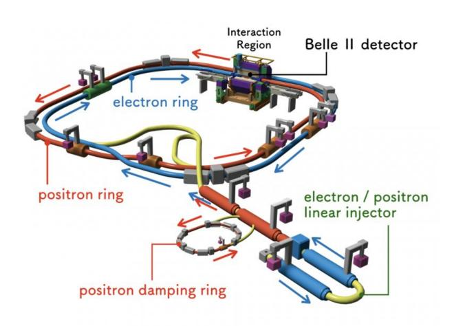
Schematic drawing of the SuperKEKB accelerator and the Belle II detector in place where particle collisions will occur. Credit: KEK
