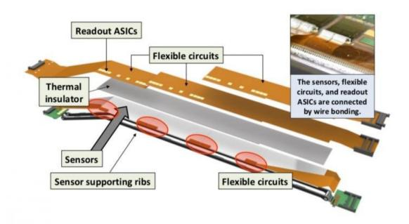
Schematic of an individual ladder. The readout integrated circuit has been placed on top of the sensor as opposed to the edge. This "chip on sensor" design was developed to minimize electric wiring and reduce noise. The red circles indicate areas where the flexible fanout circuit has been folded like origami (called the "origami concept") so that the signals on the backside of the circuit could be read out. Credit: Belle II Collaboration
