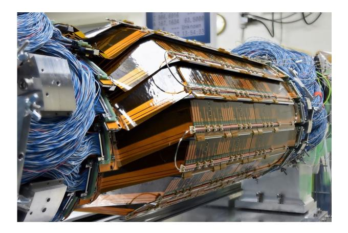
A partially completed SVD showing eight ladders assembled together like a lantern. The ladder folds inwards, becoming smaller, allowing the SVD to cover more area around a particle collision than a conventional cylindrical sensor. Credit: Belle II Collaboration
