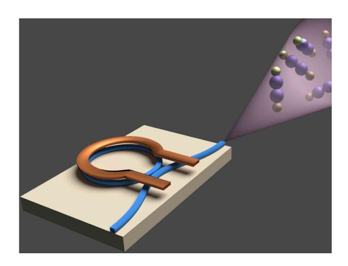
Schematic of silicon microresonator generating a frequency comb that samples molecules for chemical identification. Credit: Alexander Gaeta/Columbia Engineering
