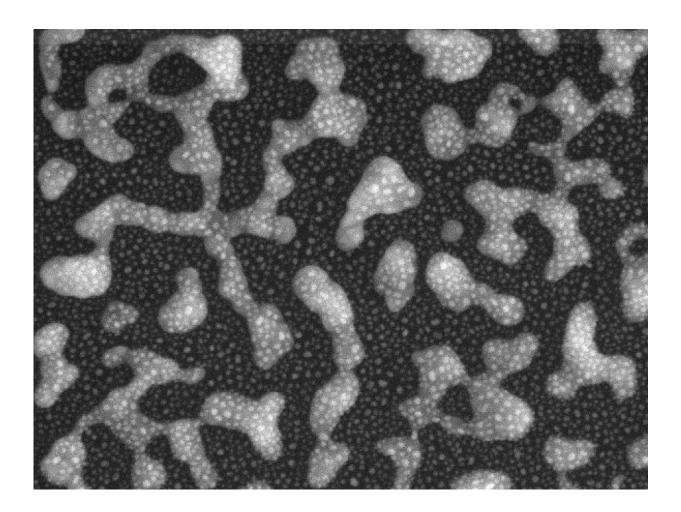
A scanning electron microscope image shows the surface of a new chemical sensing chip. The surface consists of gold nanoparticles (small bright dots) that have been deposited over silver nanoparticles (light gray regions) to form a hybrid gold-silver nanostructure. Credit: Nan Zhang
