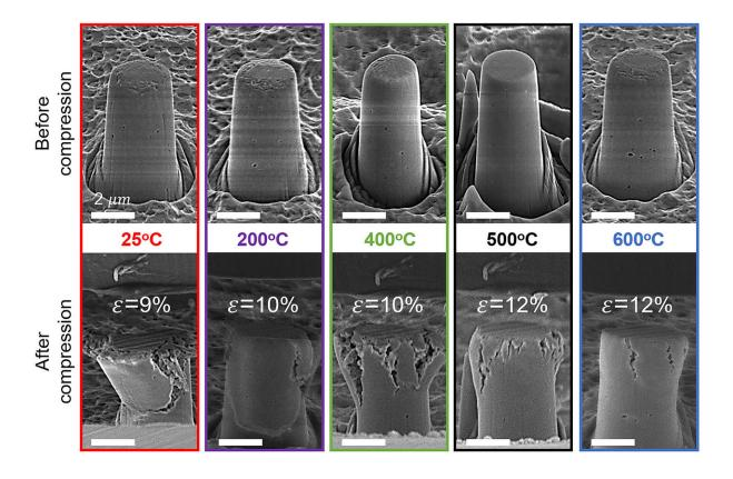
Applying an electric field to ceramics during their formation gives them the metal-like characteristics needed for sustaining heavy loads without sudden
