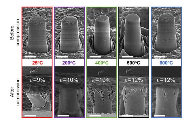
Applying an electric field to ceramics during their formation gives them the metal-like characteristics needed for sustaining heavy loads without sudden
