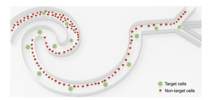
Schematic of size-based inertial cell sorting in a wavy channel unit before the trifurcated output. Differently sized biological cells can achieve distinct focusing behaviors, which thus result in effective size-based separation between target cells and non-target cells. Credit: SUTD
