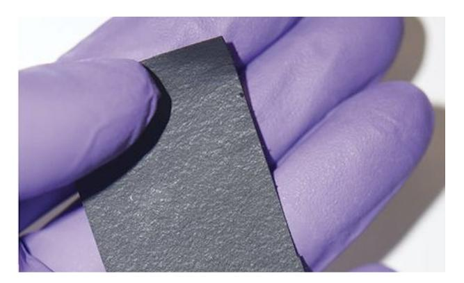
The carbon nanotube-based dough can be transformed into arbitrary shapes, such as a freestanding strip by cold rolling. Credit: Jiaxing Huang Group, Northwestern University
