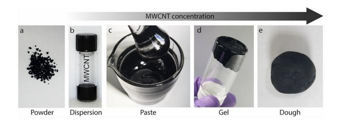
Four continuous states of (a) carbon nanotube powders in cresol-based solvent: (b) a dilute dispersion for casting thin films, (c) a thick paste for blading coating, painting, screen printing or composite making, (d) a self-standing gel for 3D printing, and finally (e) a kneadable dough that can be readily transformed into various shapes. Credit: Jiaxing Huang Group, Northwestern University
