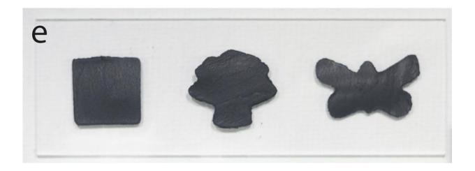
The carbon nanotube-based dough can be transformed into arbitrary shapes defined by a mold. Credit: Jiaxing Huang Group, Northwestern University
