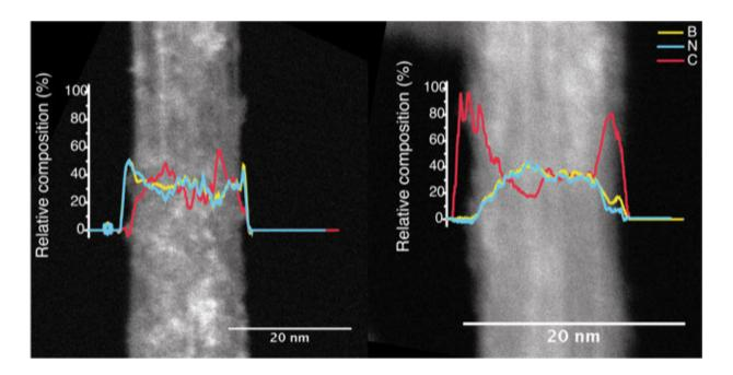
Transmission electron microscope images show a pristine boron nitride nanotube at left and functionalized nanotube at right. Rice University scientists have developed a method to make insulating boron nitride nanotubes better able to use in composite materials. Credit: Martí Research Group/Rice University
