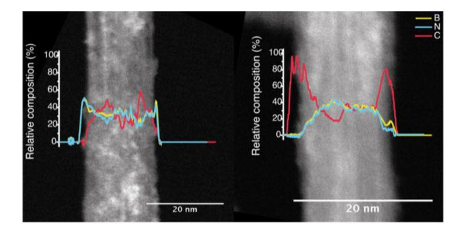
Transmission electron microscope images show a pristine boron nitride nanotube at left and functionalized nanotube at right. Rice University scientists have developed a method to make insulating boron nitride nanotubes better able to use in composite materials. Credit: Martí Research Group/Rice University
