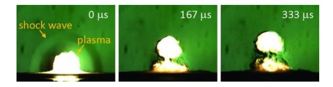
Laser-Induced Plasma: Snapshots from high-speed video showing the formation of a laser-induced plasma (8.9 mm tall) on an explosive residue; the resulting shock wave is shown in the first frame. Credit: U.S. Army
