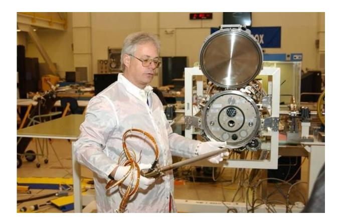
The Material Science Laboratory's Low Gradient Furnace (LGF) during preflight assembly. Credit: NASA
