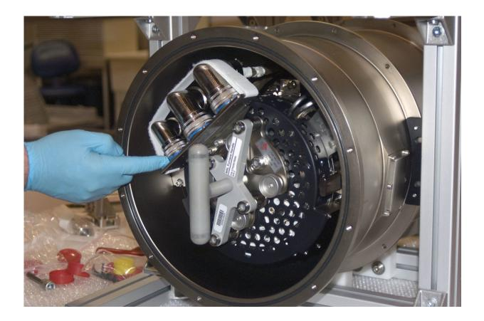
MSL's Low Gradient Furnace after installation of the flight furnace handle. Credit: NASA
