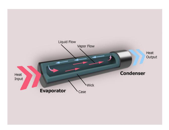
Heat pipes are devices to keep critical equipment from overheating. They transfer heat from one point to another through an evaporation-condensation process and are used in everything from cell phones and laptops to air conditioners and spacecraft. Credit: Rensselaer Polytechnic Institute
