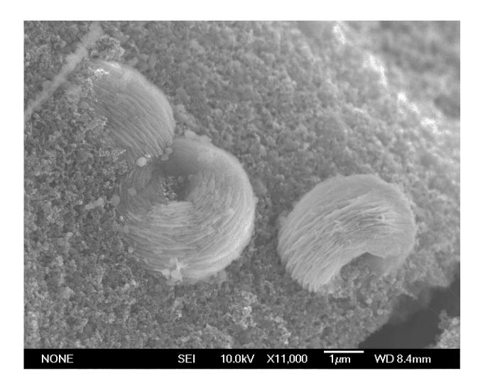
Discharged carbon cathode viewed through scanning electron microscopy by a team of researchers from Boston College and the Technical University of Denmark. The energy-storing nodules in the presence of water molecules reflects an electrolyte with promising stability. Credit: *Chem*
