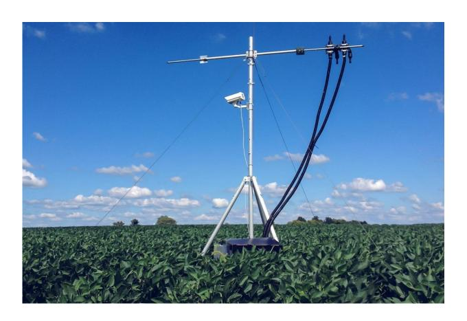
The research team used ground-mounted sensors to monitor photosynthesis in an Illinois soybean field, but the same methods could be deployed on satellites. Credit: University of Virginia
