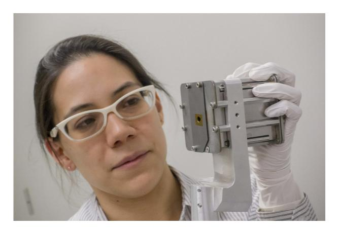
June Wicks holds a target assembly for ultrahigh-pressure laser compression experiments. The sample is mounted on the front of the box, compressed using laser pulses, and then probed by X-rays. The scattered X-rays are recorded by detectors that line the interior of the box. , June Wicks began this work as a Princeton University associate research scholar and is now an associate professor at Johns Hopkins University. Credit: Eugene Kowaluk, Laboratory for Laser Energetics
