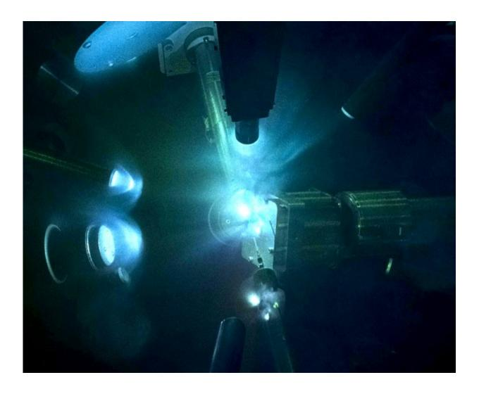
Inside the target chamber at the University of Rochester's Omega Facility, a team of researchers including Princeton University's Thomas Duffy and June Wicks use lasers to compress iron-silicon samples to the ultrahigh pressures found in the cores of super-Earths. Credit: Laboratory for Laser Energetics
