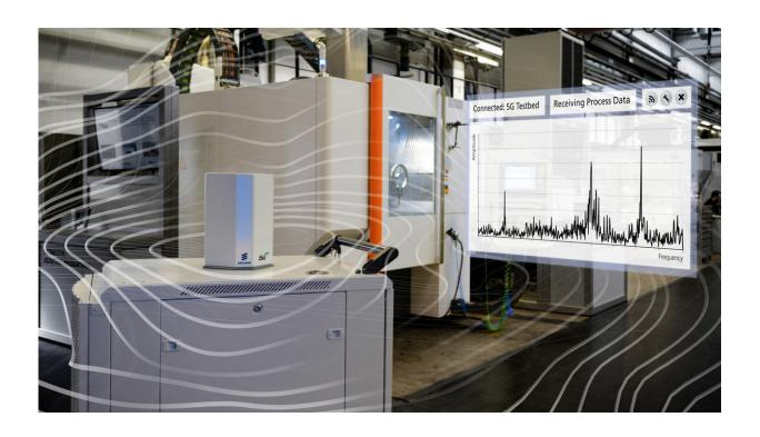
A sensor transfers the vibration spectra of the blisk via 5G with sub millisecond latency to a software. Credit: Fraunhofer IPT
