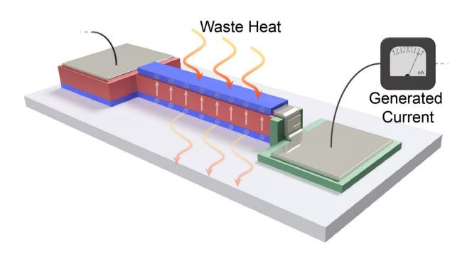
An illustration of how the thin-film device system converts waste heat to energy. Credit: Shishir Pandya
