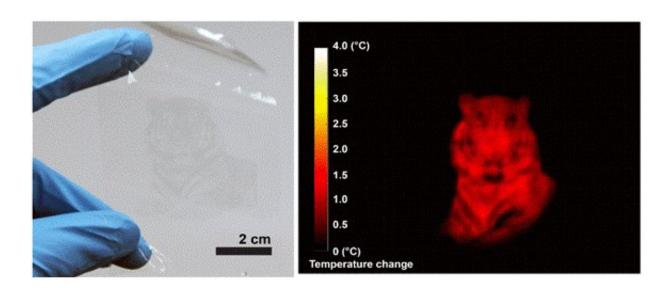
An example of an inkjet-printed thermo-plasmonic nanoparticle image on a flexible substrate in high spatial resolution over a large area (left), and remotely
