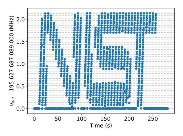
The NIST logo as spelled out by NIST's optical frequency synthesizer. The gridlinesare the expected values of the frequencies programmed into the device for thisdemonstration and the circles are the measured frequencies. The vertical axis isfrequency and the horizontal axis is the time of the measurement in seconds. Credit: Spencer/NIST
