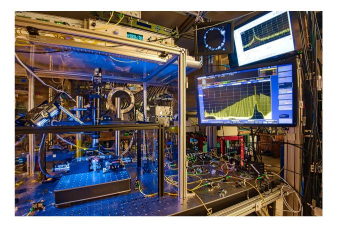
Composite photo of the testbed for NIST's chip-based optical frequency synthesizer. A key component, NIST's frequency comb on a chip, is mounted in the set-up on the lower left. A sample output of the programmable synthesizer, an optical frequency spectrum, is shown at middle-right. The synthesizer components provide for further integration into easily portable packages. Credit: Burrus/NIST
