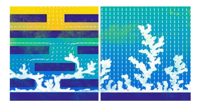
Through simulations and experiments, the research team showed that a porous membrane stifled the formation of dendrites in lithium metal batteries. Credit: University of Delaware/ Joy Smoker
