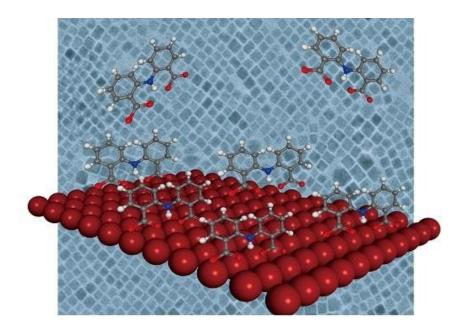
Passivating the surface of perovskite nanocrystals with IDA molecules improves their stability and their optical and electrical properties, making them useful for optoelectronic devices. Credit: KAUST
