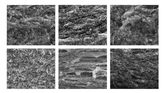
The conductive felt is made of stacks of interwoven silver-coated copper nanotubes filled with a stretchable silicone rubber (left). When stretched, felt made from more pliable rubber is more resilient to small tears and holes than felts made of stiffer rubber (middle). These tears can be seen in small cavities in the felt (right). Credit: Matthew Catenacci
