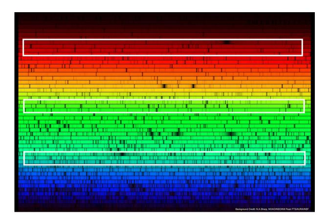
HERMES, the new spectrograph built at the AAO, uses volume phase holographic (VPH) gratings to provide various optimized spectra in blue, green and red light and a fourth band in infra-red light. HERMES spectra allows astronomers to study the chemical makeup of stars to understand their formation and evolution. A spectrum of the Sun shows many dark features because of various chemical elements in sunlight. Credit: N.A. Sharp, NOAO/NSO/Kitt Peak FTS/AURA/NSF.
