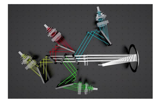
A schematic of the HERMES instrument showing the light path of how star light from the telescope AAT is split into four different channels. Credit: The Australian Astronomical Observatory (AAO)
